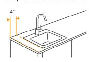
Use a small sink that fits into a 24" cabinet. Make sure to have at least 4" between the sink and the edges of the countertop to ensure sturdy construction.
