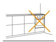
An oven next to a wall disrupts work flow by limiting available work space, and it'll put the wall at risk from heat and cooking stains.
