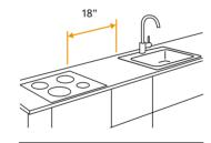
To have a good preparation area, try to squeeze in at least 18" of work space between the countertop and the sink.
