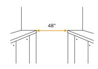
02 Make sure that the distance between opposite rows of cabinets is wide enough for doors on both sides to be opened at the same time, and for multiple cooks to move around safely.
