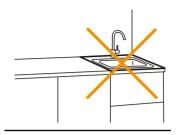
Placing a sink next to a wall or at the end of a row of cabinets disrupts work flow by limiting available work space.
